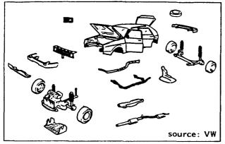
Fig. 13 Modular design of an automobile
