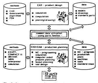
Fig. 5 Integrated system for product design and production planning
