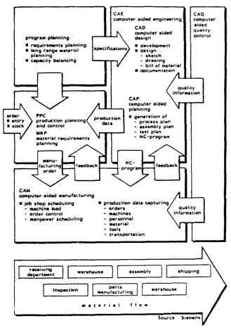
Fig. 4 CIM-computer integrated manufacturing
