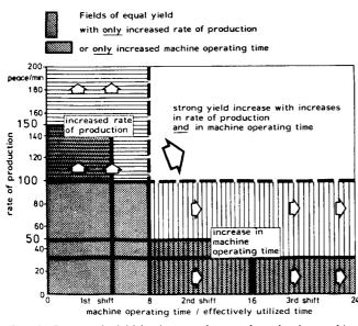
Fig. 7 Increased yield by increased rate of production and/or machine operation time
