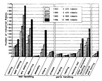
Fig. 9 Application fields for industrial robots in Germany
