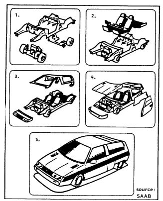
Fig. 14 Module concept for a final car assembly
